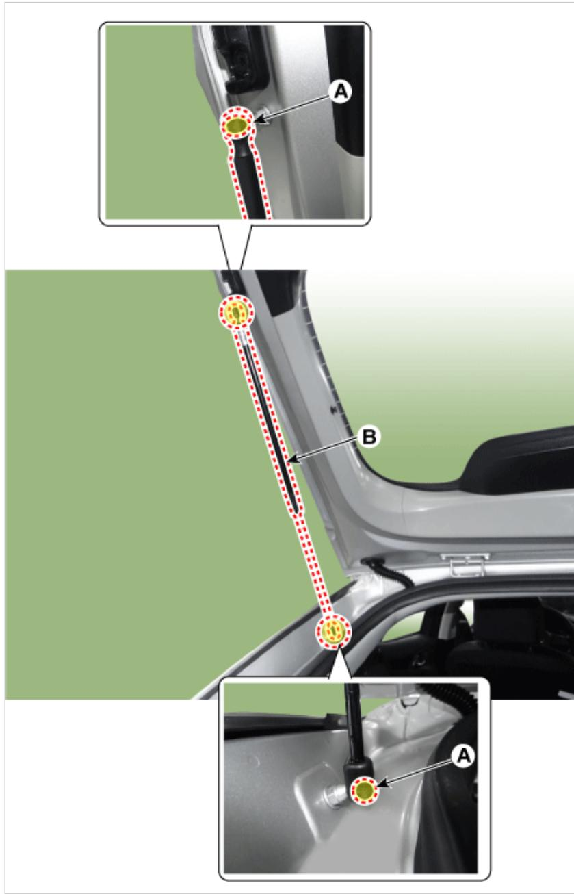
2. Push the socket of the lifter into the bracket for installation.
